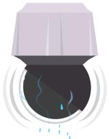
The Sharpdome technology includes Axis' unique Speed Dry function that helps to provide sharp images in rainy weather. It also simplify dome cleaning, allowing for more efficient methods such as high pressure cleaning. With the Speed Dry function activated, the dome vibrates at high speed. It breaks the surface tension of the water and removes the drips.
