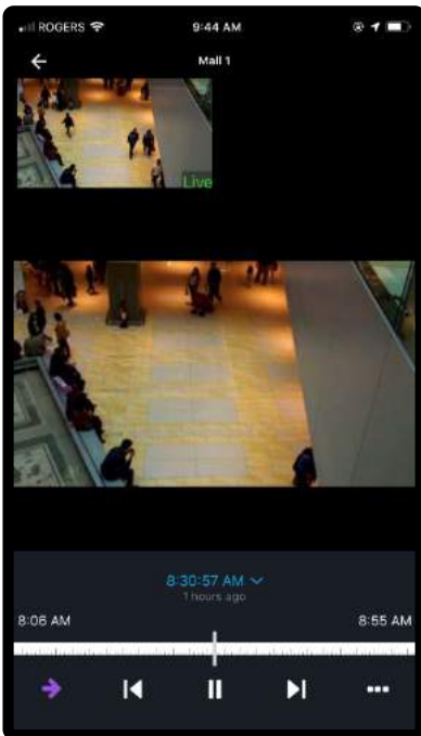
Omnicast video: Live and playback video can be accessed. Actions such as PTZ controls, add bookmark, save snapshot & iris/focus control are available at the click of a finger. Stream video from a smartphone or other mobile devices to Security Center
